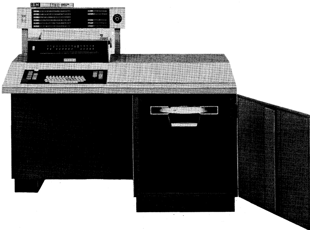
IBM 1131 Central Processing Unit with disk drive
